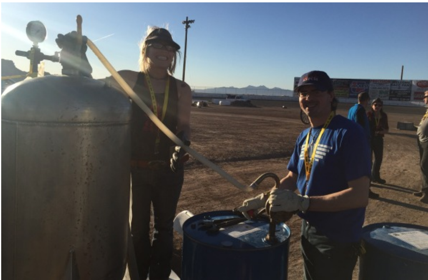
Coloring agents are mixed into methanol fuel by rolling the barrel back and forth. Then the contents are pumped into a pressure vessel that will force them out through nozzles in the Egg. Above: JDV and Caroline. Below: Denise and Liam. Photo credits: Denise, Caroline.
