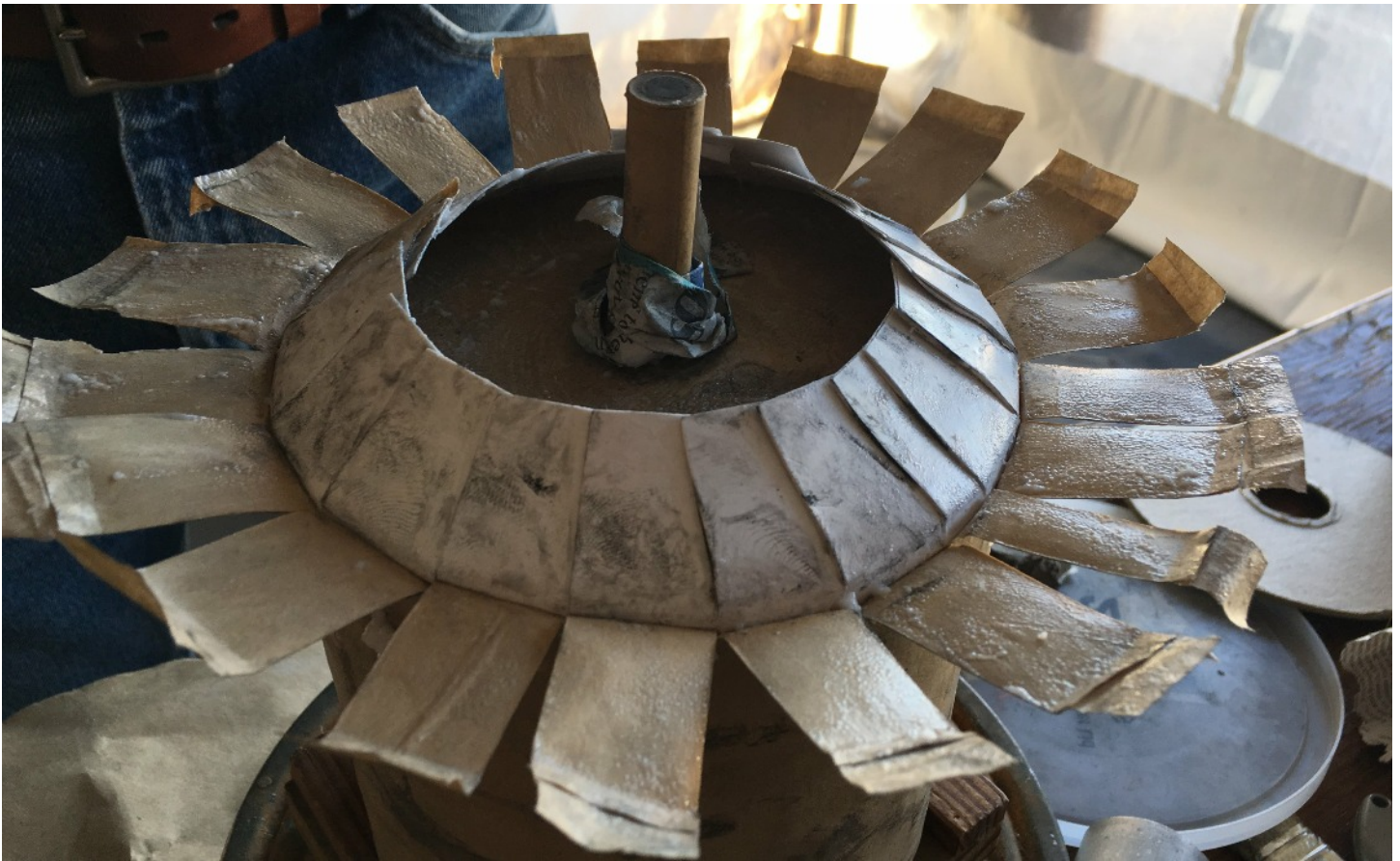
The thin card that formed the shell body is carefully folded in and pasted down to the inner end disk
